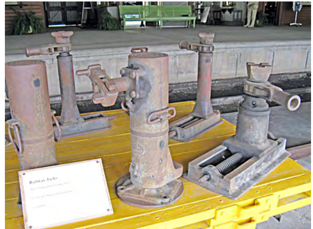
A selection of railway jacks used for lifting rail, wagons and locomotives. [lz 0332]
