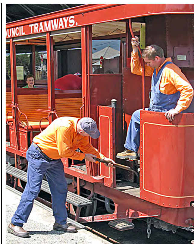
Adding fuel to the Purrey's firebox is a two person task. The use of Blair Athol coal and coke ensures steady running and relatively little smoke.
