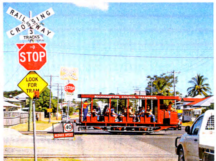
The crossing signs are there to warn motorists! The Purrey steam tram is running in Denison St and crossing Cambridge St. The nearest track is the line into Archer Park station. Australian rail safety requirements mean that the tram crew are dressed in high visibility clothing, rotating beacons are attached to both tram ends and there are also electric horns with back-up compressed air horns. The original conductor and driver bells are still used for inter-crew communication. ALL: ANDY PLUNKETT
